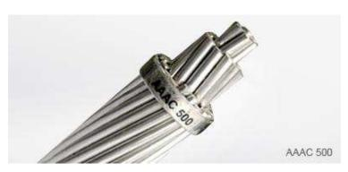
distribution and in cases where high strength-to-weight ratio is required. It has a good corrosion resistance due to being composed out of aluminum alloy wires only, minimum conductivity of 52% IACS, high breaking strength per weight and normal creep values. AAAC has the highest strength per weight among all bare overhead conductors.
